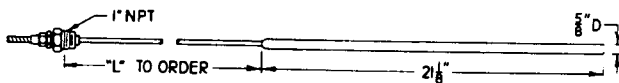
Style No. 706—Plain Bulb with 1" Union Connection and 1/4" OD Bendable Extension. Dimension "L" must be specified.
