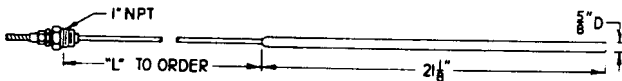
Style No. 706—Plain Bulb with 1" Union Connection and 1/4" OD Bendable Extension. Dimension "L" must be specified.
