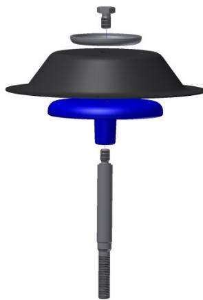
Remove the old diaphragm and replace with a new one. Place the diaphragm plate (3) on the diaphragm, then turn the diaphragm over and place the diaphragm ring on the other side, apply Loctite 270 to the thread on the bolt then screw this into the diaphragm plate by hand.
