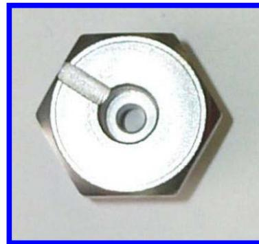
Figure 1 Top View of Seat with SLR
