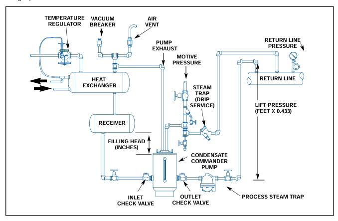
To efficiently drain condensate in a closed system, the receiver should be horizontally located a minimum of twelve inches above the pump to allow for sufficient condensate collection. The receiver must be sized to provide the minimum condensate capacity required to prevent equipment flooding. The receiver may be either an ASME coded tank or a length of large diameter pipe. A safety relief valve may be required. Consult factory for capacity when a steam trap is utilized after the pump.
