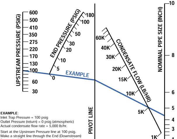
Make a straight line through the End (Downstream) Pressure of 0 psig and stop at the pivot line. From that point, make a straight line through the Condensate Flow Rate of 5,000 and stop at the
