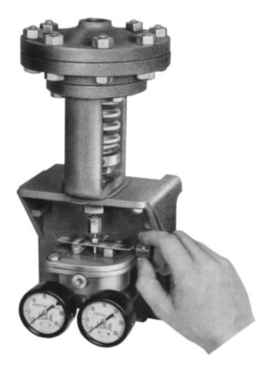
PDAP and PRAP Pressure Pilots are also available for applications requiring valve positioners, volume boosting or other relays or receiver controllers with various modes of control. Both types may be used as controllers or transmitters.
